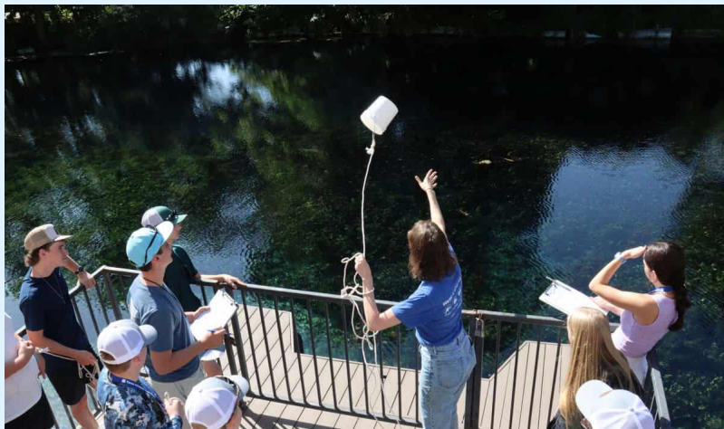
Ambassadors were trained how to properly collect and measure for dissolved oxygen, pH, turbidity and total dissolved solids.
